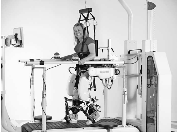
Fig. 2. The Lokomat gait rehabilitation robot with Lokolift body weight support system (Photo courtesy of Hocoma AG, Switzerland)
