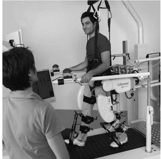
Fig. 1. Human subject walking in the Lokomat gait rehabilitation robot (Photo courtesy of Hocoma AG, Switzerland)
